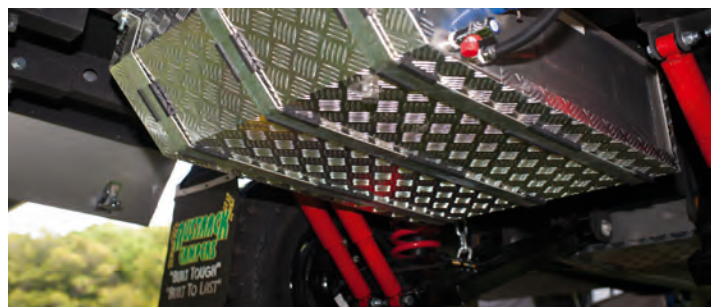
Water storage: 120 L stainless steel underfloor water tank with aluminium tank guard & 12 volt pump plumbed to kitchen. 50L stainless steel underfloor water tank with aluminium tank guard & 12volt pump plumbed to cold water shower system.
