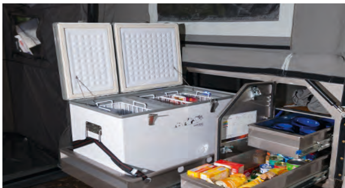
Fridge: Fridge slide, 980 (L) x 540 (W) x 580(H) mm with tie down points & ventilation fan.
