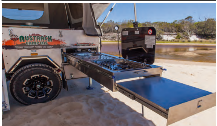
Slide out stainless steel kitchen: cutlery & utility drawer, tap, sink & 3 burner smev stove & extension bench.
