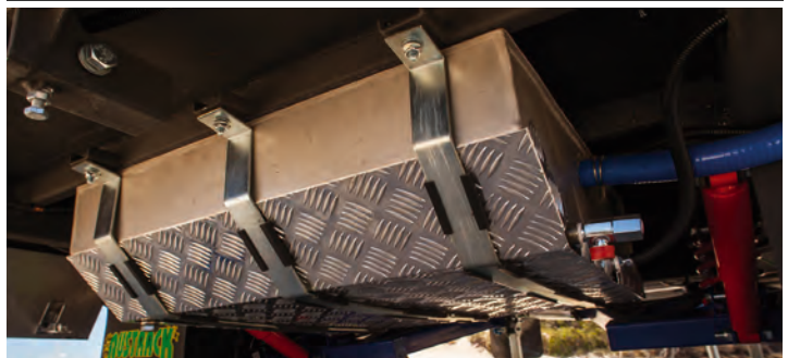
Water storage: 100 L stainless steel underfloor water tank with aluminium tank guard & 12 volt pump plumbed to kitchen and ensuite.
