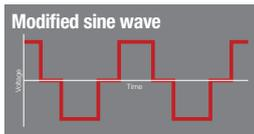
Appliances running on a modified sine wave need more power and will produce more heat. For this reason, appliances designed to run on a pure sine wave will overheat if run on a modified sine wave.
