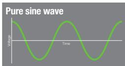
The change in a pure sine wave is smooth and gradual, ensuring the correct functioning and efficient operation of high end electronic equipment.
